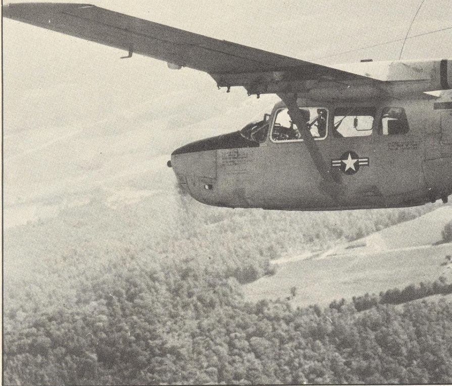
The modest variety of stores and/or armament which an O-2 might go out with can be listed on the side panel just ahead of the forward lower window.
